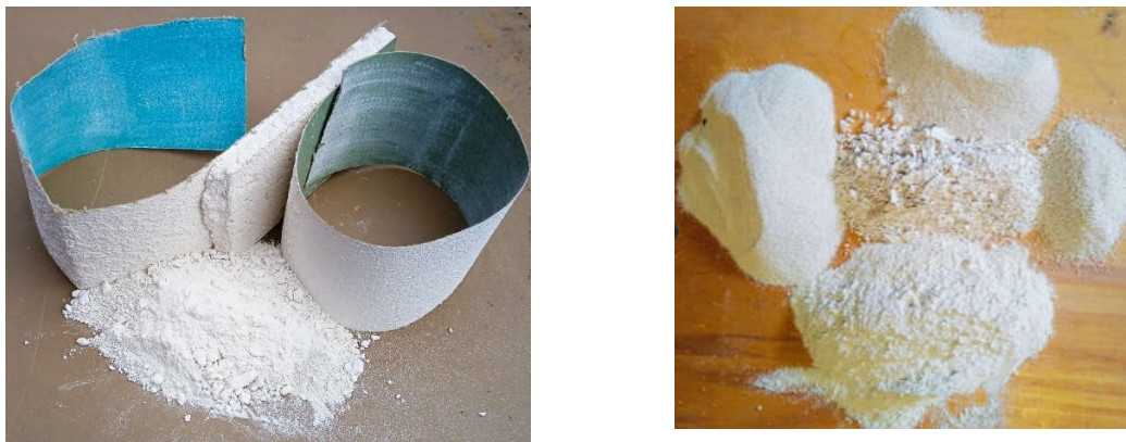
Fig.5. Crushed gypsum component of gypsum board
