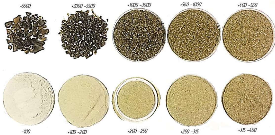
Fig.4. Distinguished size classes ( \mu\text{m} ) of brown container glass
