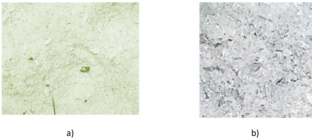
Fig. 3. Crushed sheet glass waste at the discharge gap: a – 0 mm, b – 10 mm
